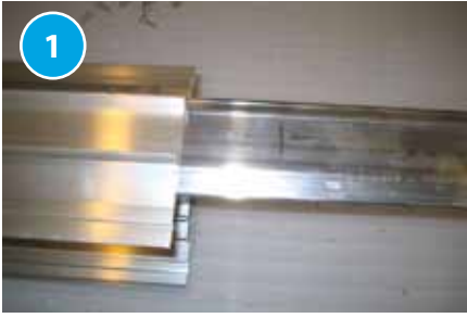
Slide the aluminium joiner half way into the body of one ridge.
