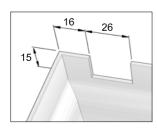
Cut out a section 26mm wide by 15mm high for the top fascia section **XGUTF-AL1** to fit into. This is done 16mm from the outer edge as shown.
