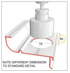
Using a 75mm diameter hole saw cut a hole through bottom section of aluminium gutter fascia (XGUTF-AL3) using the central die line, and set <a href="mailto:90mm">90mm</a> forward from the wall end of the gutter fascia
