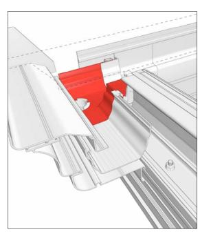
Using standard lead flashing procedures, ensure flashing is extended to seal off corner as shown above (dotted line).
