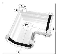
Prep 90° External Bend (XYR-935) by cutting a hole on the intersection of the two centre lines as shown using a 60mm hole saw.
