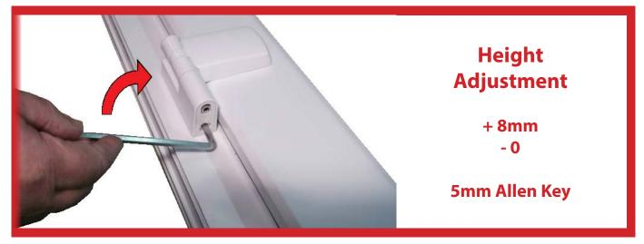
Rotate the Allen Key clockwise to give the required height setting Ensure that the weight of the door is evenly distributed across all hinges
