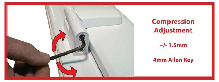
Rotate the Allen Key clockwise or anti-clockwise to give the required compression setting Ensure compression is evenly distributed across all hinges Note: In rotation positive "click" positions are felt - (2 in each direction from the central position)
