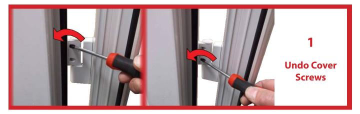
Open the door to access the Cover Retaining Screws. These are self retaining screws therefore to release the cover the screws must be completely uncrewed. However, the screws do not come out.
