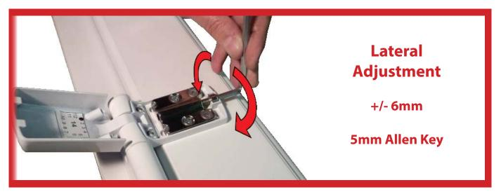
Rotate the Allen Key clockwise or anti-clockwise to give the required lateral setting Ensure even distribution across all hinges
