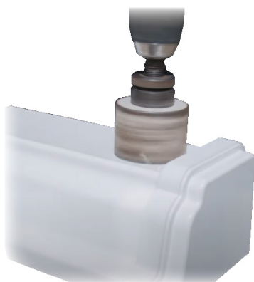
52mm diameter drill / hole saw
