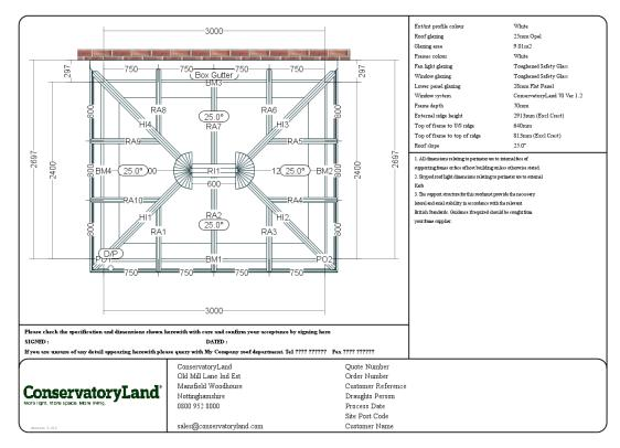
Refer to your roof plan that you used to build the main roof structure. The numbering for your Internal Pelmet parts are the same as the roof ring beams.
