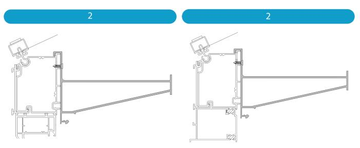
Fit the Faux Orangery Support Brackets first. (Brackets for the corners of your roof are cut down versions).
