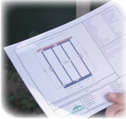
Using your roof layout plan, identify the Ring Beam which is the first component to be fitted. Ring Beam and wall plate components are usually labelled with a 'BM' number.
