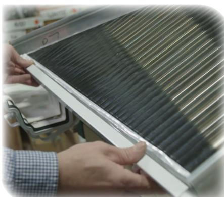
**The breather tape at the end of the sheet must not be covered or blocked in anyway.**
