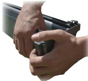
To fit the Stop Ends there is no need to remove the clips on the Stop End. Clip one end of the Gutter into the Stop End and then push the other end up to the stop under the clip. You will need to use some force to do this.
