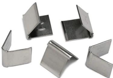
To firmly hold the flashing in place prior to sealing, it is good practice to use flashing clips (also known as hall clips). These are readily available from most DIY stores, builders merchants, or your local Eurocell branch. These push into the chase line in the mortar and are easily installed. Nylon flashing clips are also available at DIY stores.
