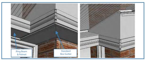
The above drawing shows Internal Pelmet on the Ring beam only, butted up to the box Gutter. Unless you have requested not to have it, Pelmet will be supplied for both the Box Gutter & Ring Beams.
