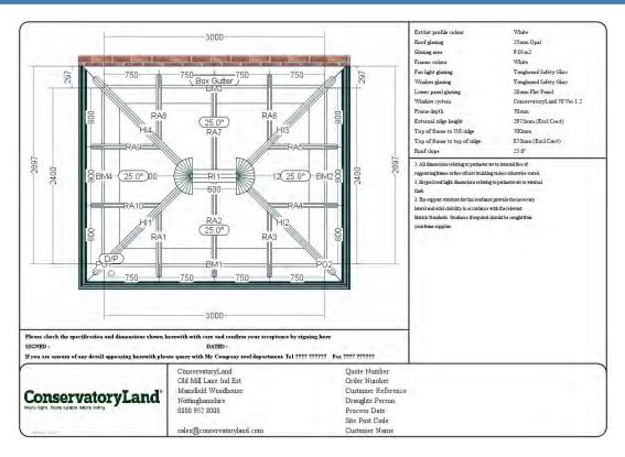
Refer to your roof plan that you used to build the main roof structure. The numbering for your Internal Pelmet parts are the same as the roof ring beams.
