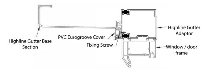
Once the Highline Gutter Adaptor and Ring Beams are in position, hook the High line Gutter Base section to the Highline Gutter Adaptor as shown, and fix at 300mm centres using the screws provided.
