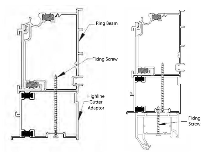
Fix the Highline Gutter Adaptor to the Ring Beam by screwing up through the adaptor into the Eaves Beam at 500mm centres. Move the Highline Gutter Adaptor & Ring Beam into position onto the frames and fix up through each frame into the adaptor using the 70mm self drilling screws. Use 2 per frame / door sash, or a maximum of 500mm centres. Do not fix within 150mm of any corner weld on your frames.
