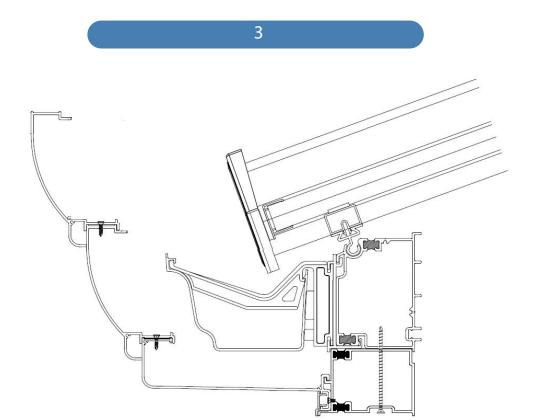
Fit the Highline Gutter Section 2
