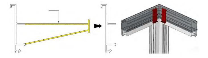
See below for the correct positioning of the brackets in the corners of your conservatory roof.
