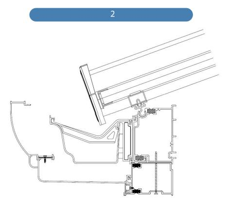
Next fit the Highline Gutter Section 1
