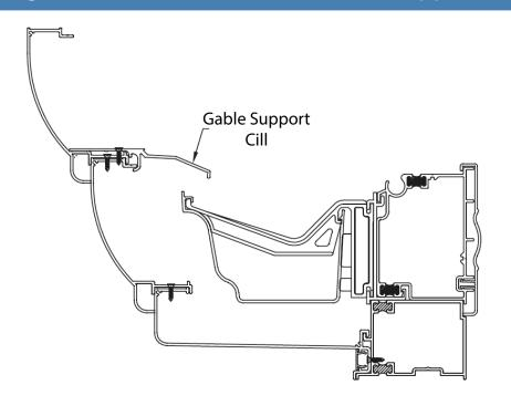
To ensure any rainwater is directed into the standard gutter, locate and fix the gable support cill into the second section of Highline Gutter. This will act as a cill.
