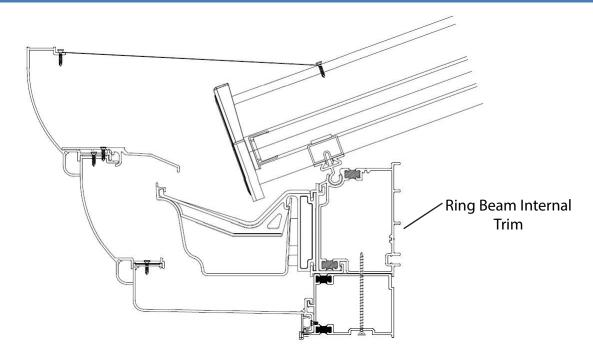
If the conservatory you have ordered does not have any Internal Pelmets, there are just the Ring Beam Internal Trims and Ring Beam Cover Joints to install. Please see the Installation Guide you used for the main roof structure. If your conservatory has Internal Pelmets, please see the following guide.
