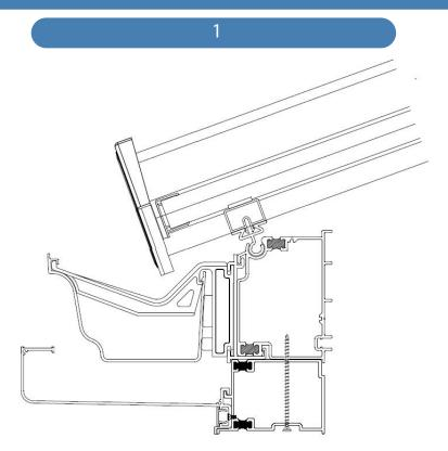
Fit the Highline Gutter Base
