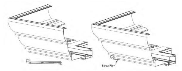
Fix the bottom section of the casting through the underside into the high line gutter base.
