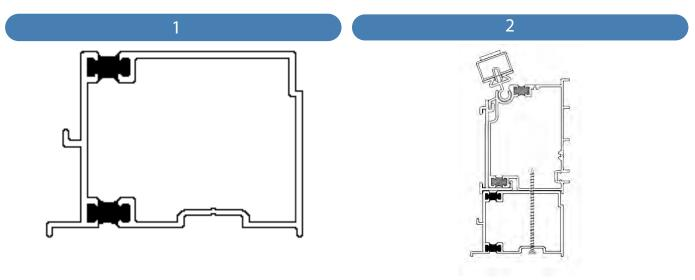
Identify the Highline Gutter Adaptor, And fix this to your ring beams using the fixings supplied. This MUST be done first to be able to install your Decorative Highline Gutter.
