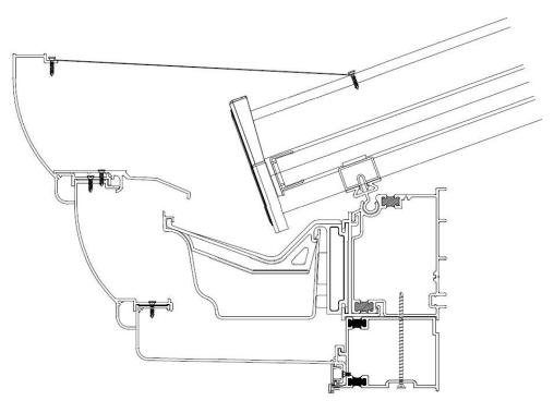
Finally fit the Tie Wires
