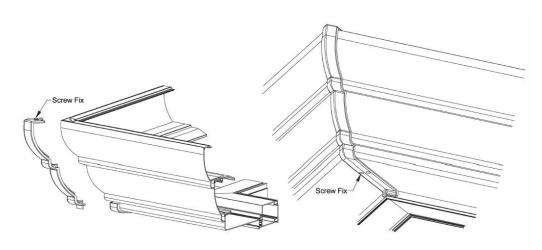
Fix the top part of the casting, fixing down through the top into the highline gutter section.
