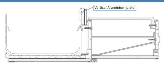
Where there is a Box Gutter cut out, the Pelmet will fit in exactly the same way as previously described for Ring Beams & standard Box Gutters. The only difference is the Ring Beam is replaced with a different component that is just a narrower version of a Ring Beam, designed to hold the vertical Aluminium plate that sits on top of it.
