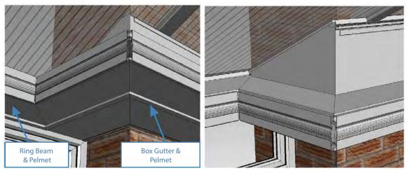
The above drawing shows a Box Gutter cut-out with the Internal Pelmet fitted.
