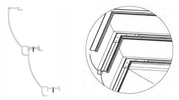
Fix the second section of Highline Gutter to the first at 300mm centres with the screws provided. Again use cleats on the corners or any straight joints to the inside of the gutter as shown above right, and as the previous step.
